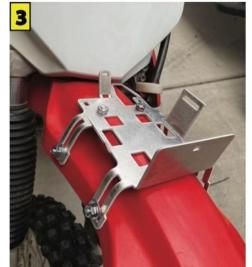
Your BITD timing transponder and RacingTraX tracker cannot both be mounted onto the same fender.
